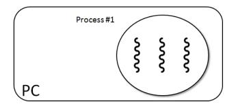
Figure 2: Single process with multiples threads
